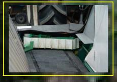
Padded web and powered lower plough deliver fruit to the self-contained trailer. This helps to reduce damage and removes leaves from the sample.
